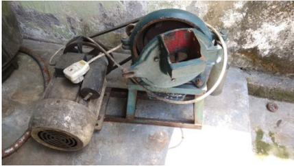
Gambar 4. Disk mill lama
